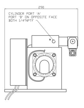
DC ELECTRO-HYDRAULIC POWER UNIT FOR ECS
