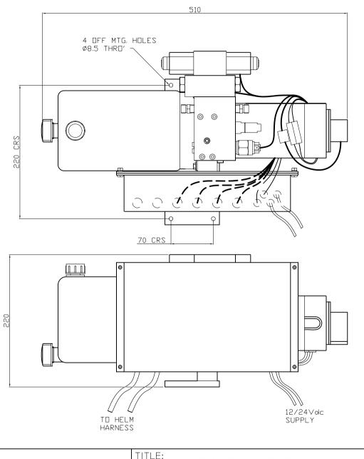
CURRENT DRAW: (24vDC UNIT) TYP. 35-40A MAX. @ 1500PSI (100BAR)
